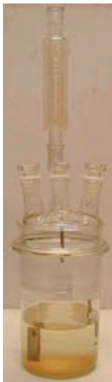
Figure 37.4.2.2: Exposure receptacle with reflux condenser
